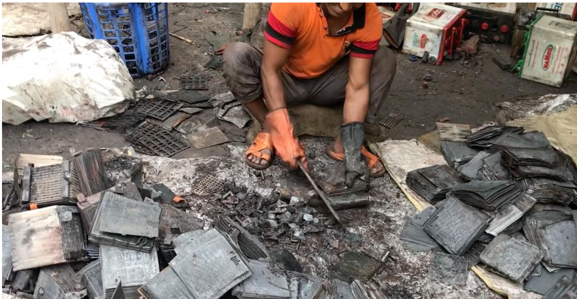
Figure 1. Manual disassembly of lead-acid batteries.
