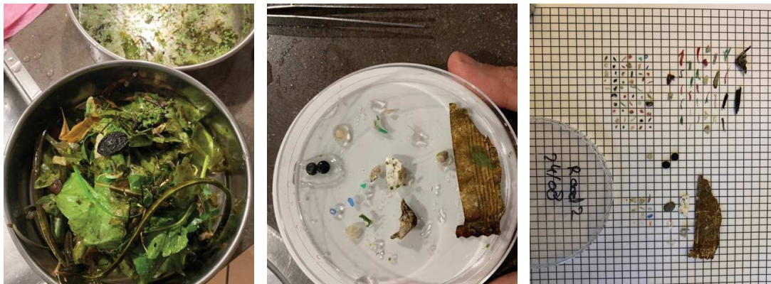
Figure 3. Sample in sieve with organic matter (left), plastic pieces removed to petri dish (middle), and plastics divided in groups on laminated grid-paper with sample name (right).
