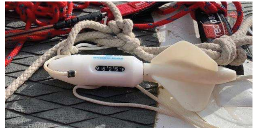
Figure 1. Flowmeter on SUP board.
