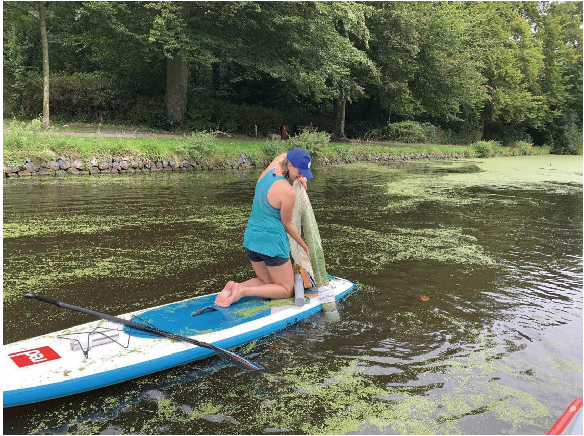
Figure 2. SUP-Trawl is taken out of the water. The net is full of duckweed which makes the analysis more difficult. Reduce the sampling time should that be the case.
