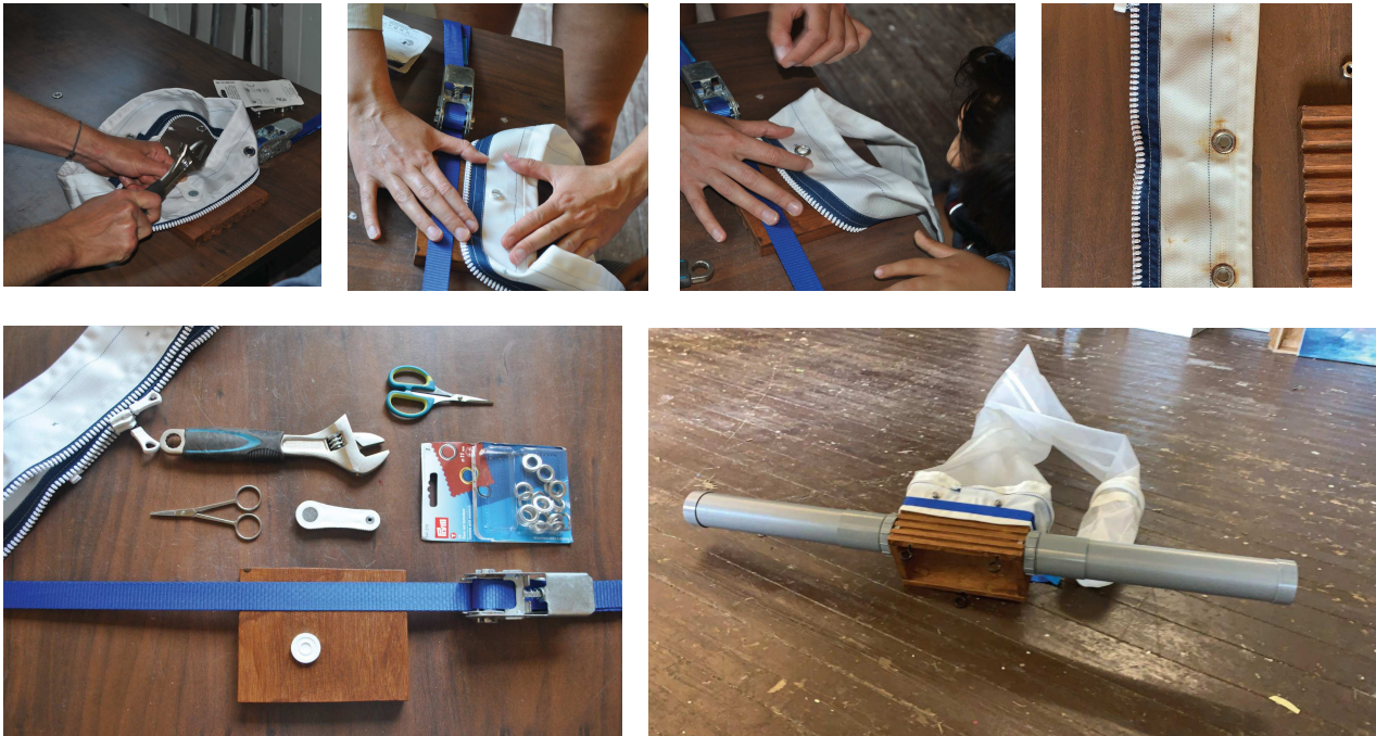
Figure 3. Pressing grommets through nylon webbing (top 4 pictures), Materials (bottom left), and final results of the frame with grommets en tension strap (bottom right).
