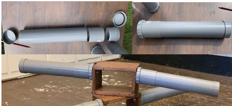
Figure 1. The parts of the floating wings (left), the assembled wings (right), and the wings attached to the frame (bottom)
