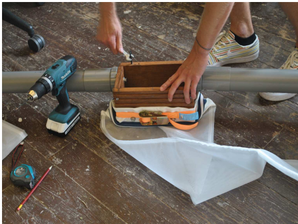
Figure 4. screwing in the screw eyes in pre-drilled whole in the frame (left) and the frame with rope attached through the eyes and dettached wings for transportation(right).
