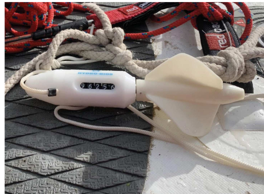
Figure 2. The double amount of materials for the net (left) and the flow meter on a SUP board (right).
